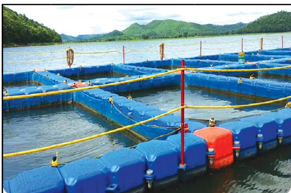
HDPE Floating Pontoon Cubes used for suspending Nylon Net Cages for fish culture
